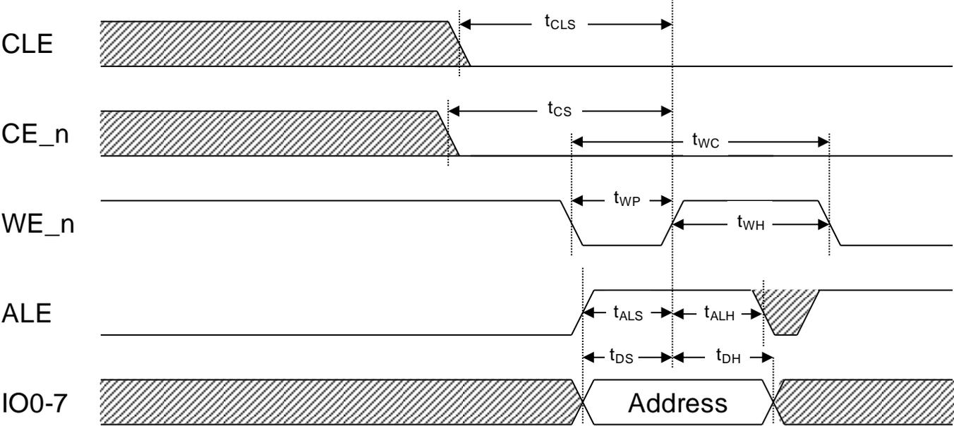
Figure 57 Address latch timings
