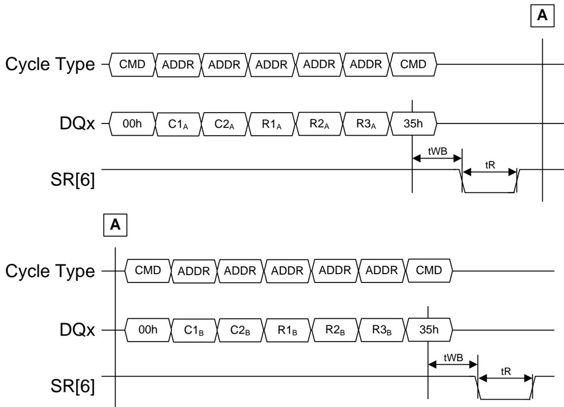
**Figure 135 Non-multi-plane Copyback Read timing for multi-plane Copyback Program**
