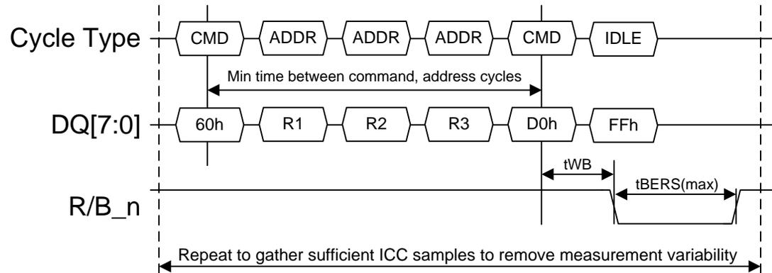
**Figure 146 ICC3 measurement procedure**
