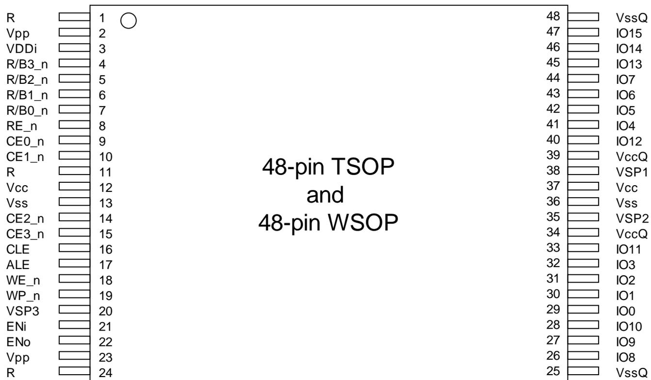
**Figure 3** 48-pin TSOP/WSOP pinout for 16-bit data access
