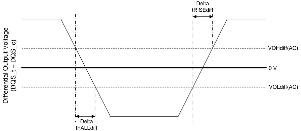
**Figure 43** tRISEdiff and tFALLdiff Definition for Output Slew Rate, NV-DDR2/3 (differential)
