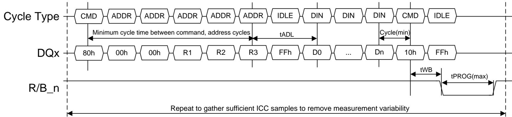
**Figure 145 ICC2 measurement procedure**
