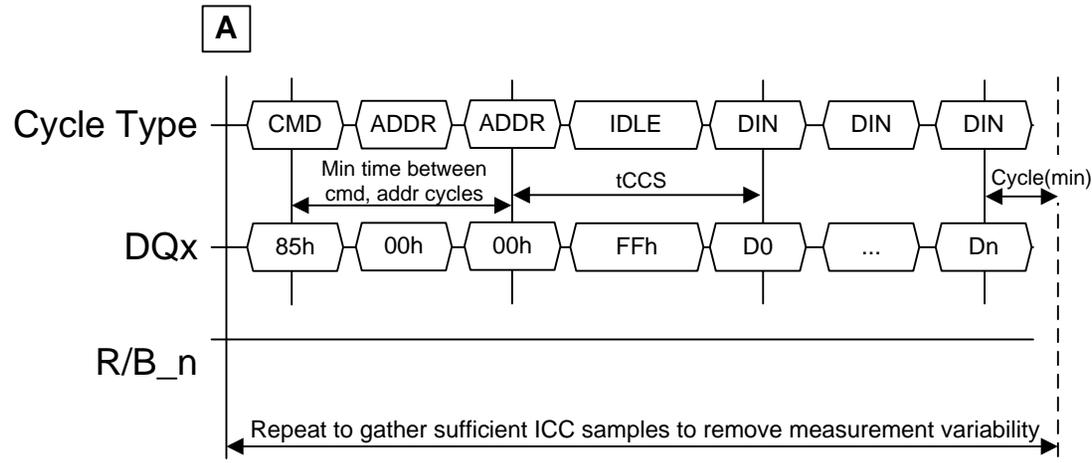
Figure 148 ICC4W measurement procedure
