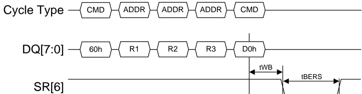
**Figure 92 Block Erase timing**
