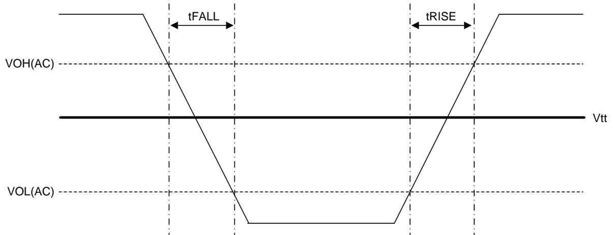
**Figure 42**  $t_{RISE}$  and  $t_{FALL}$  Definition for Output Slew Rate, NV-DDR2/3 (single-ended)
