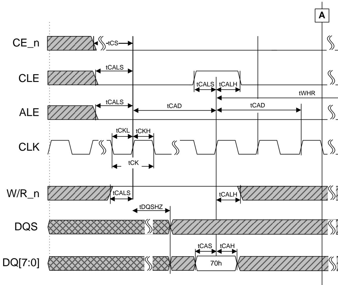
Figure 70 Read Status including  $t_{WHR}$  and  $t_{CAD}$  timing requirements
