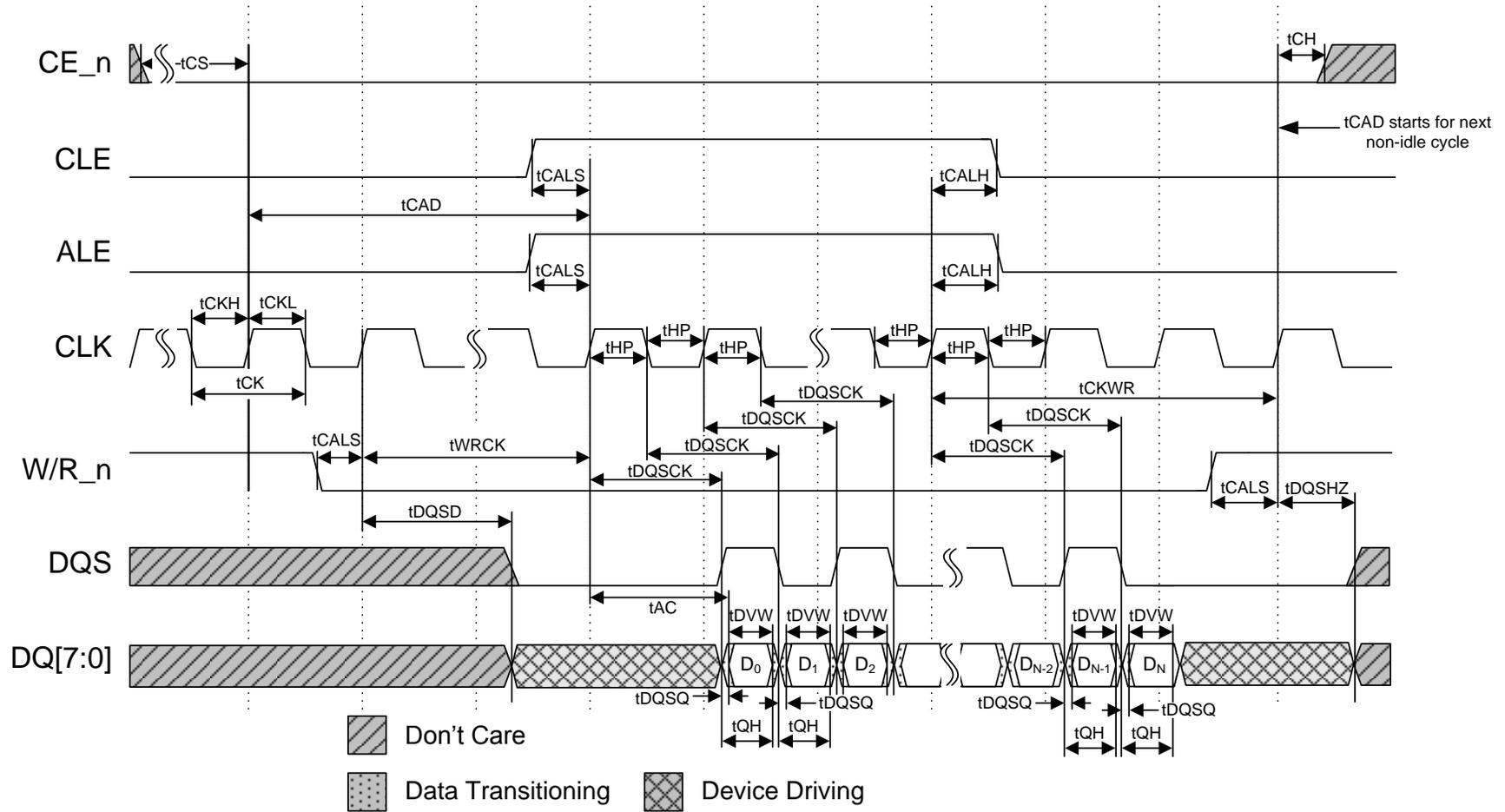
Figure 68 Data output cycle timing
