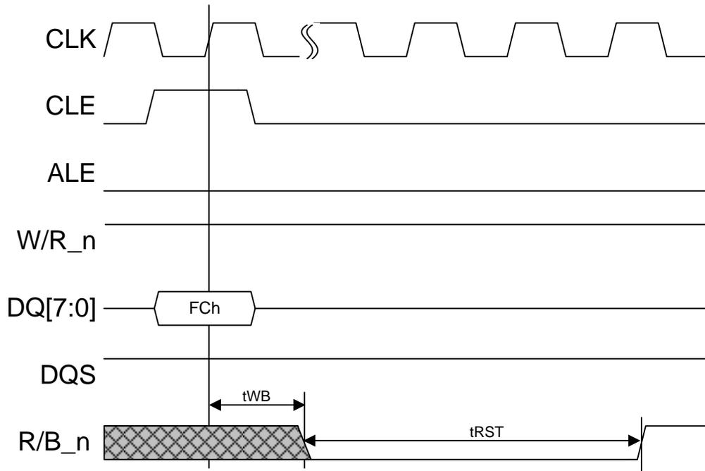
Figure 83 Synchronous Reset timing diagram
