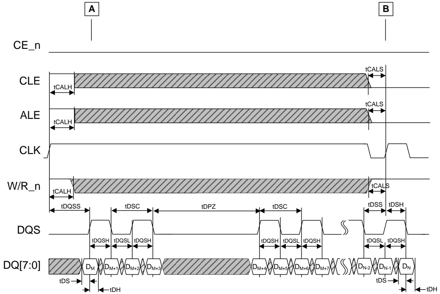
**Figure 67** Data input cycle timing, CLK stopped with data pause
