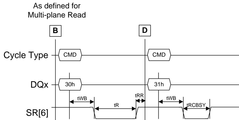
**Figure 142 Multi-plane Read Cache Sequential command issue timing**
