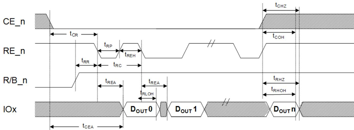
Figure 60 EDO data output cycle timings
