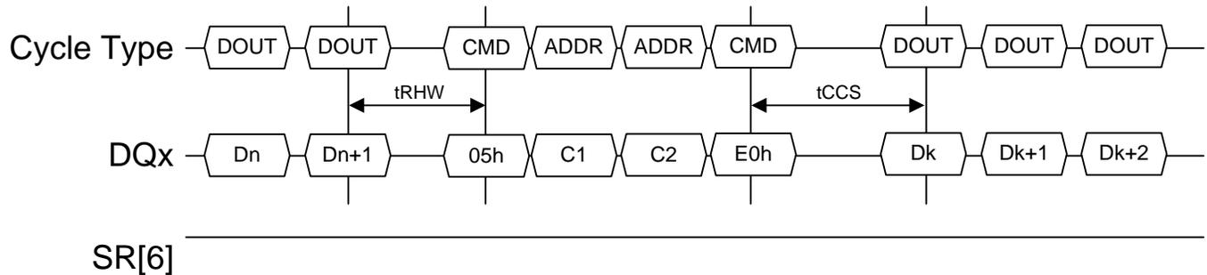
**Figure 110 Change Read Column timing**
