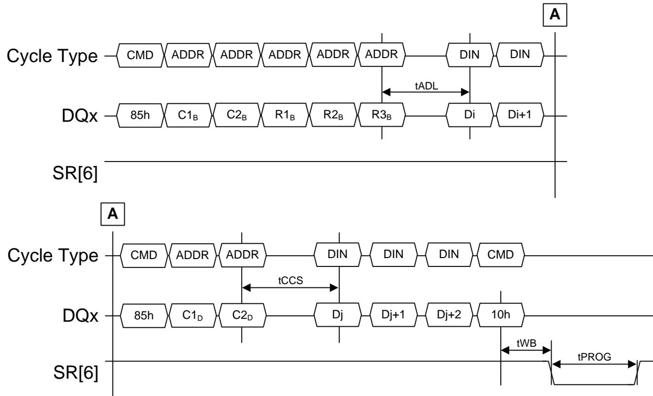
**Figure 107 Copyback Program with data modification**
