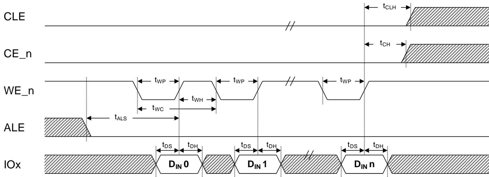
Figure 58 Data input cycle timings
