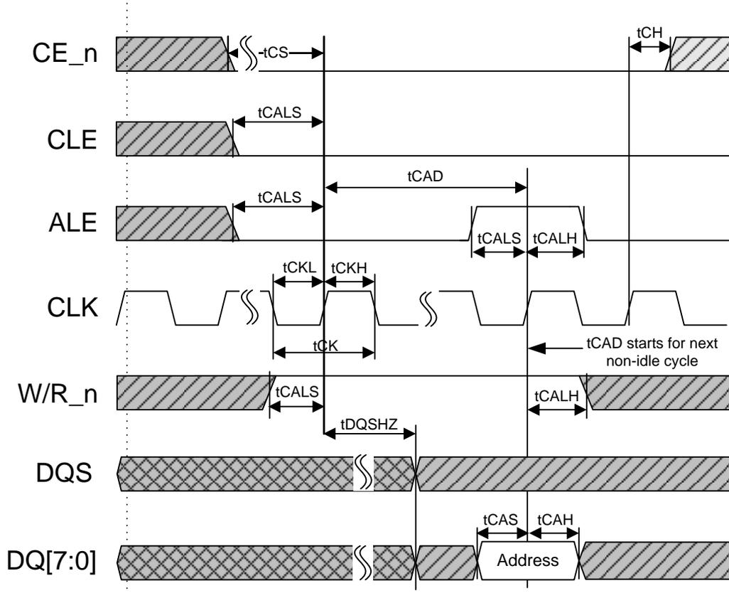
Figure 64 Address cycle timings
