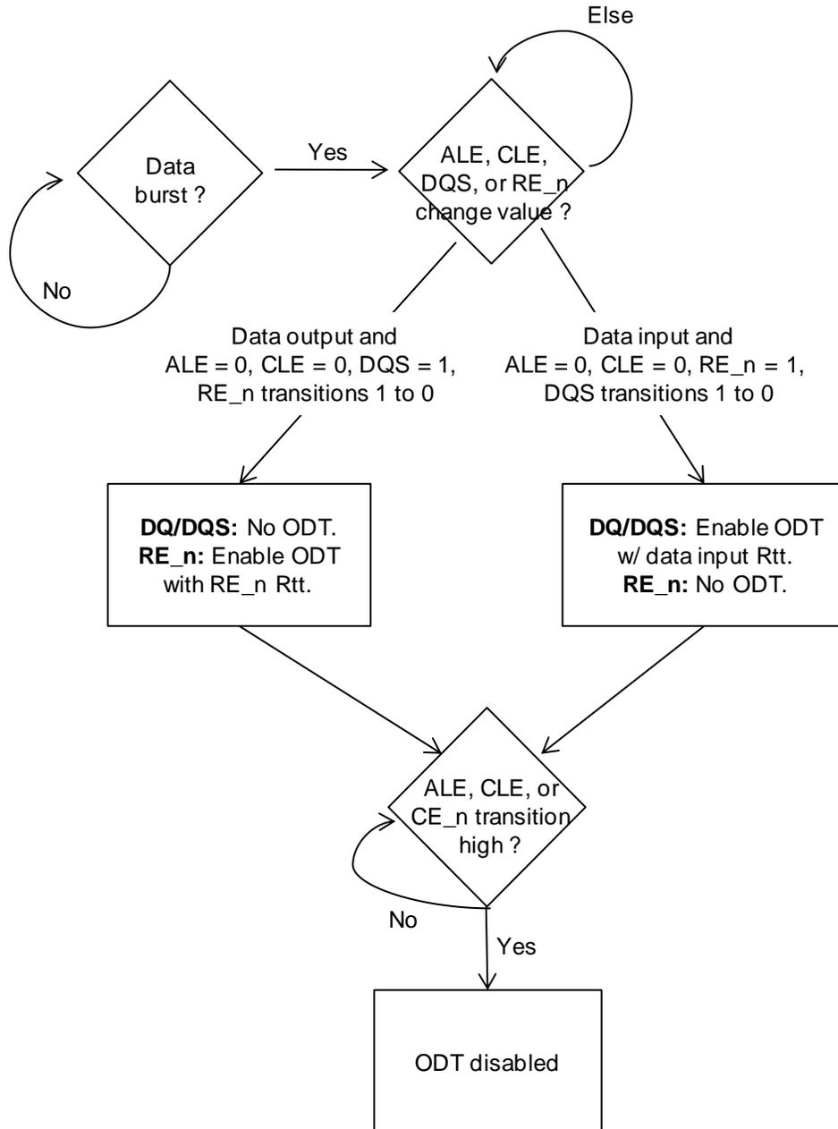
**Figure 51 Self-termination only ODT Behavioral Flow**
