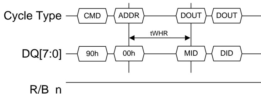
**Figure 86 Read ID timing diagram for manufacturer ID**
