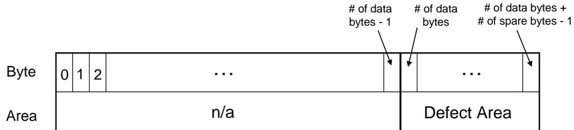
Figure 35 Area marked in factory defect mapping
