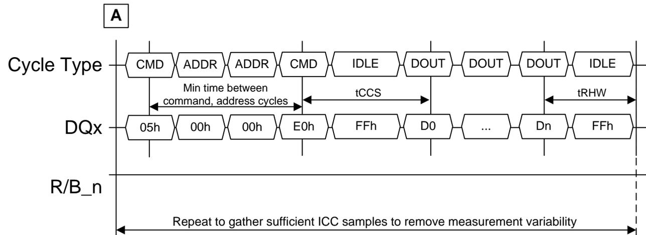
**Figure 147 ICC4R and ICCQ4R measurement procedure**
