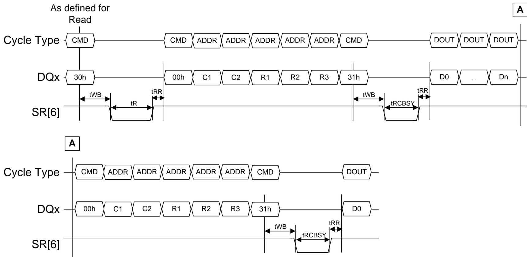
**Figure 100 Read Cache Random timing, start of cache operations**
