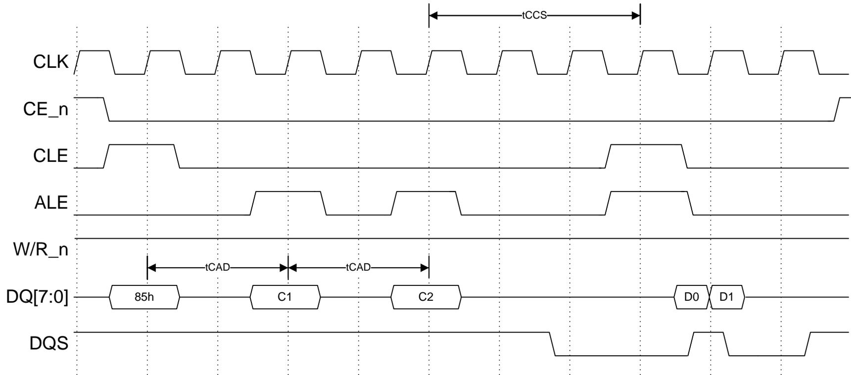
**Figure 80 NV-DDR data interface command description**
