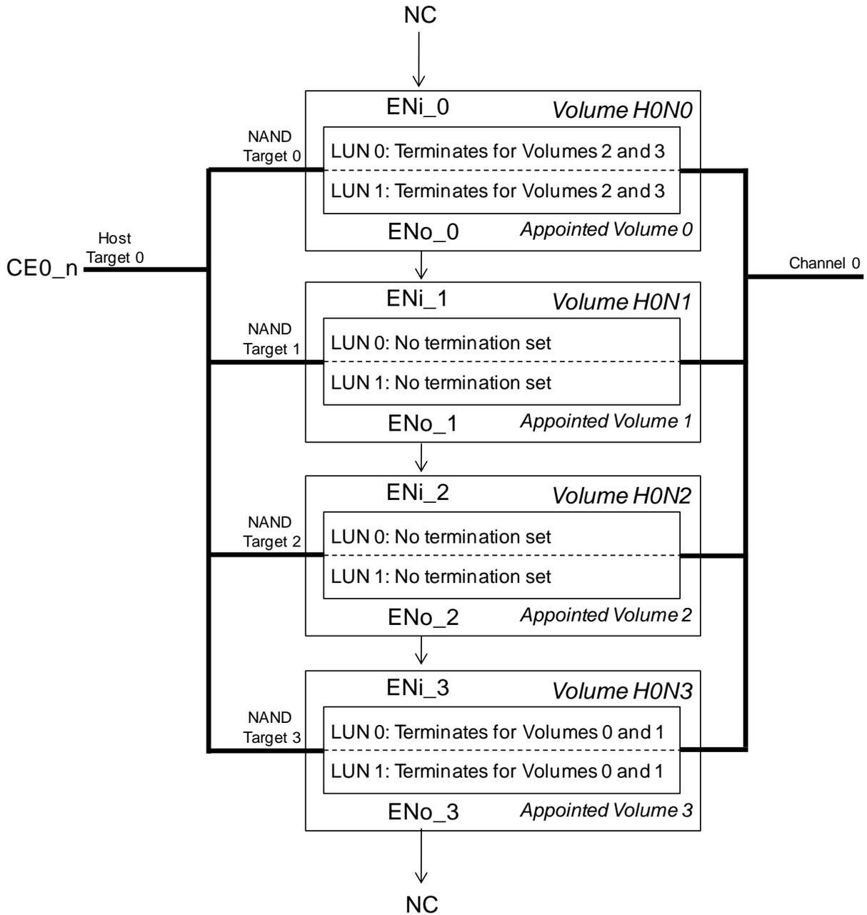
Figure 55 Example: Parallel Non-Target ODT
