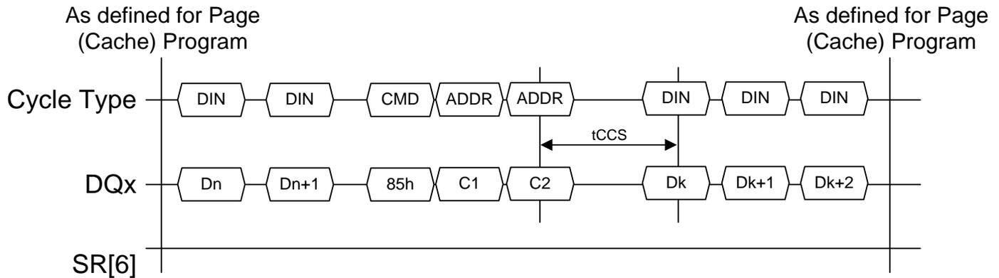
**Figure 113 Change Write Column timing**
