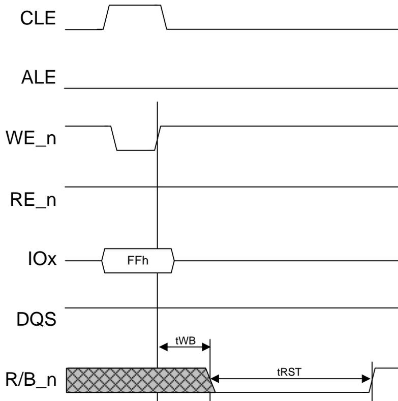
Figure 82 Reset timing diagram
