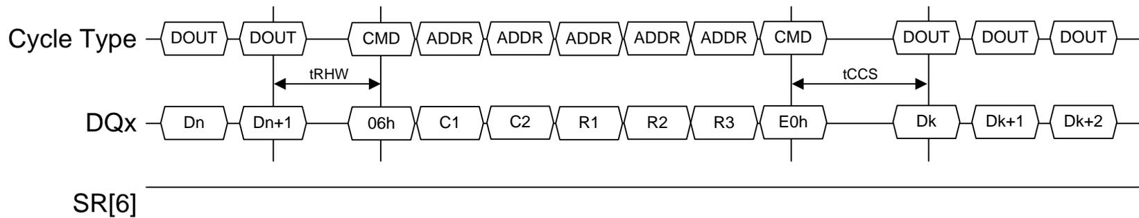
**Figure 111 Change Read Column Enhanced timing**
