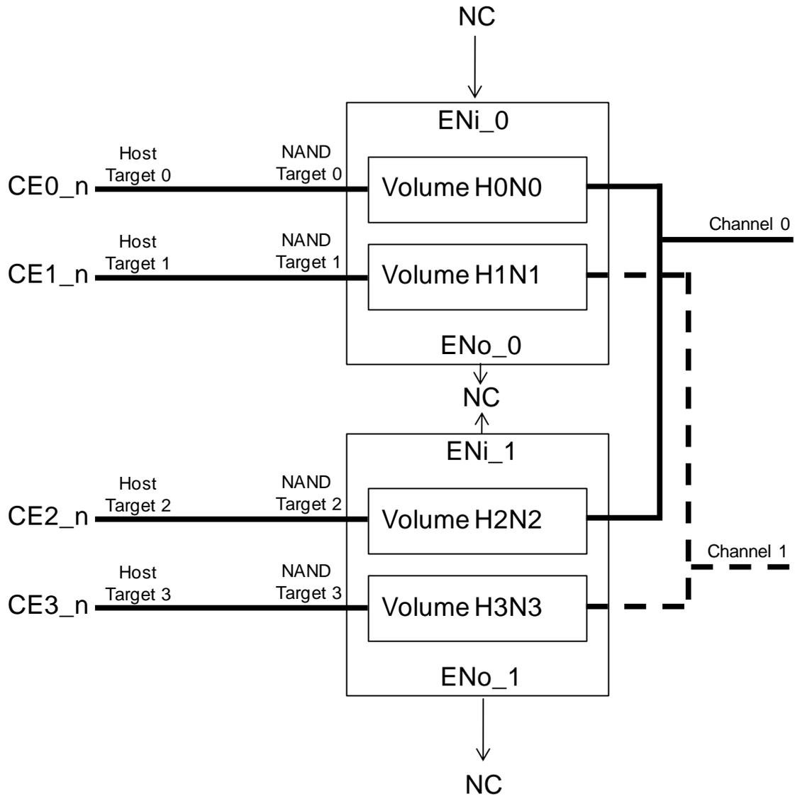
Figure 30 Discrete CE<sub>n</sub> per package topology
