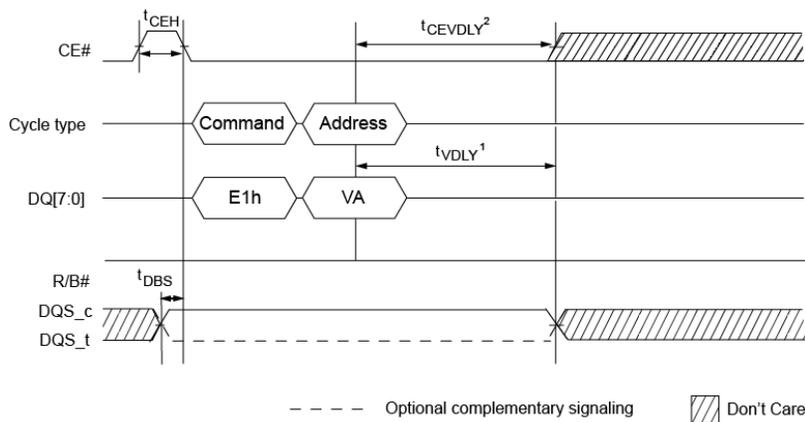
**Figure 115 Volume Select timing diagram**
