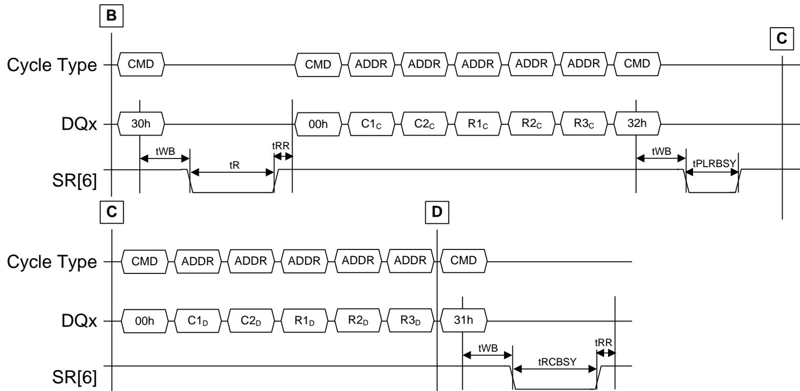
**Figure 143 Multi-plane Read Cache Random command issue timing**
