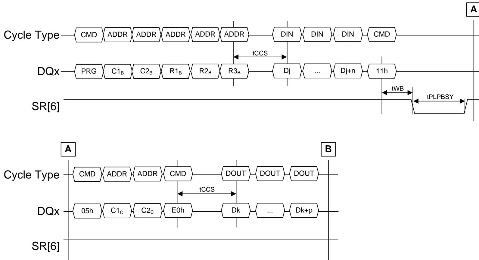
**Figure 108 Small data moves, data modification**
