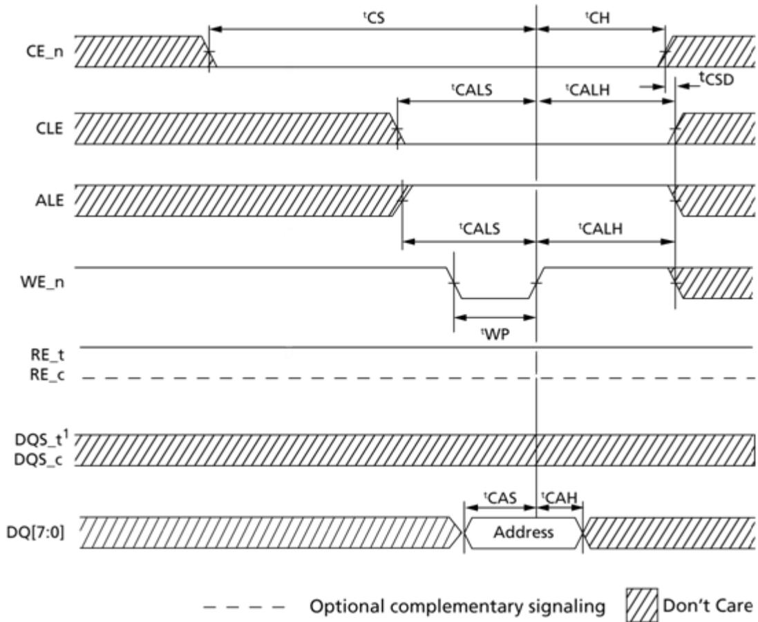
**Figure 73 Address cycle timings**
