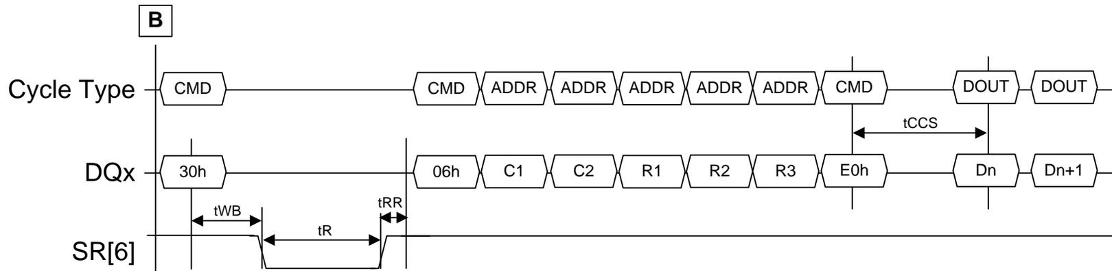
**Figure 141 Multi-plane Read data output timing, continued from command issue**
