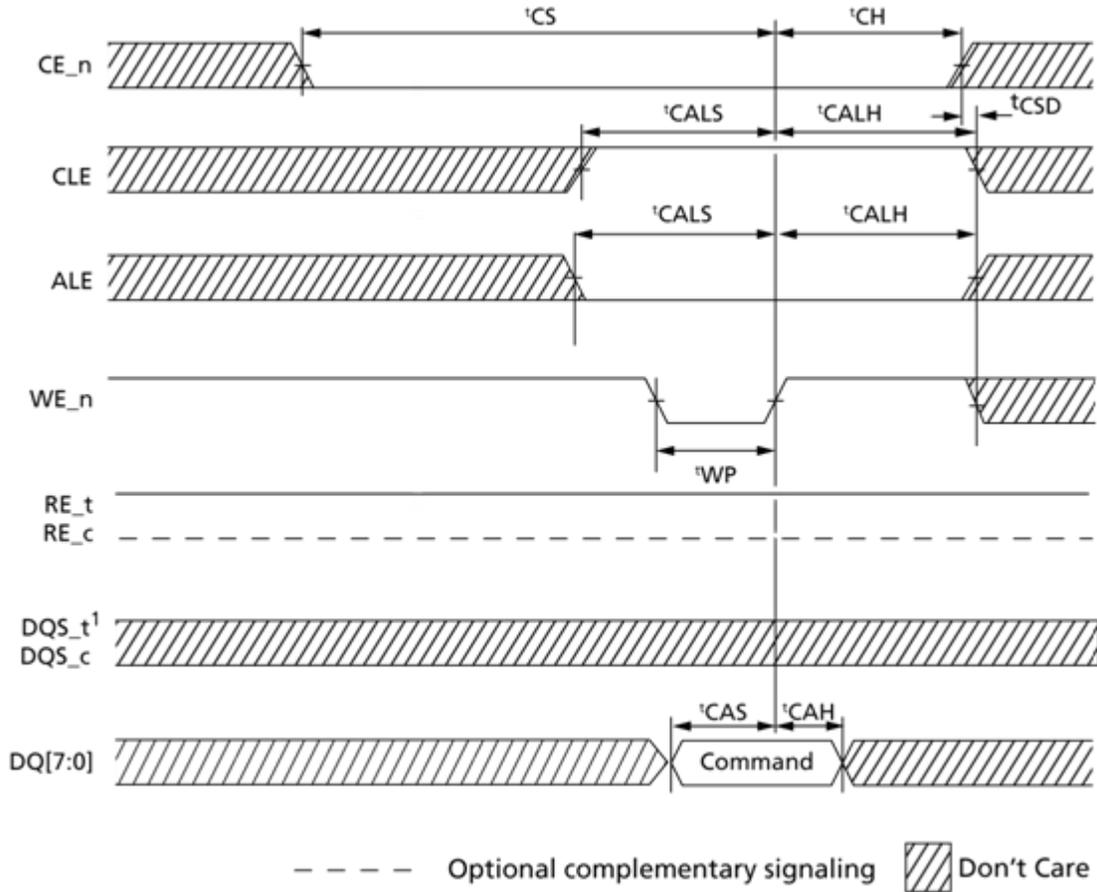
**Figure 72** Command cycle timings
