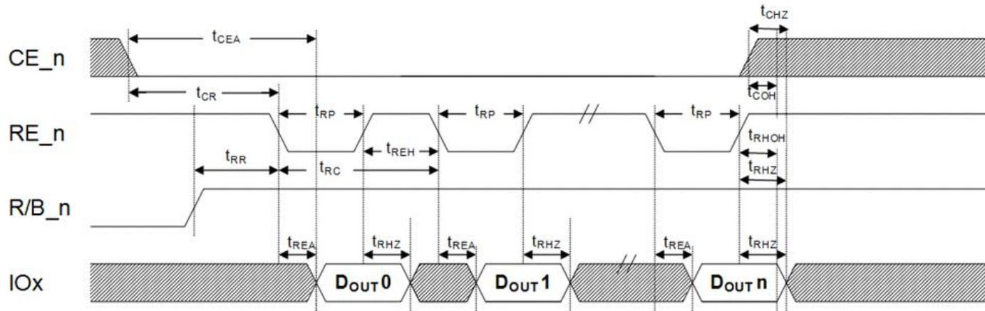
Figure 59 Data output cycle timings
