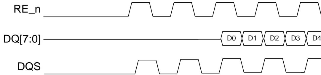
**Figure 50 Warmup Cycles for Data Output**
