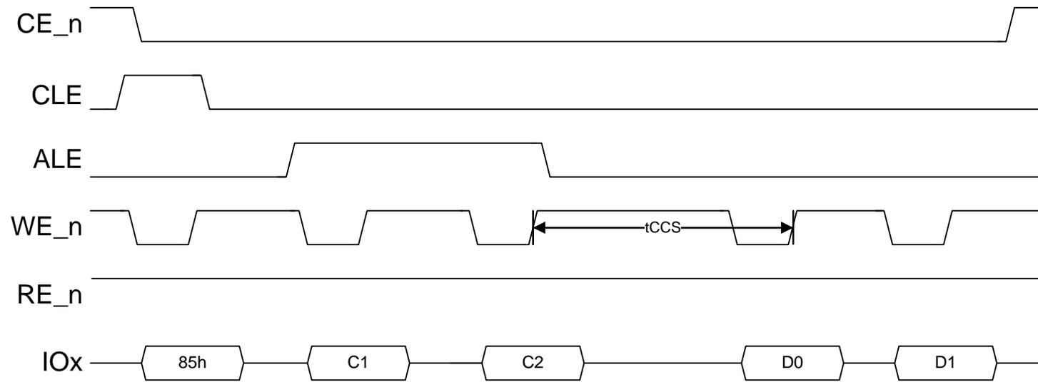
**Figure 79 SDR data interface command description**
