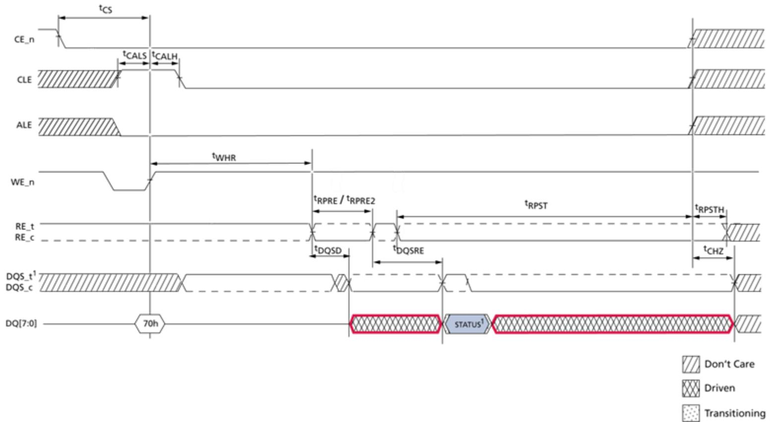
Figure 96 Read Status command using NV-DDR2/3 data interface
