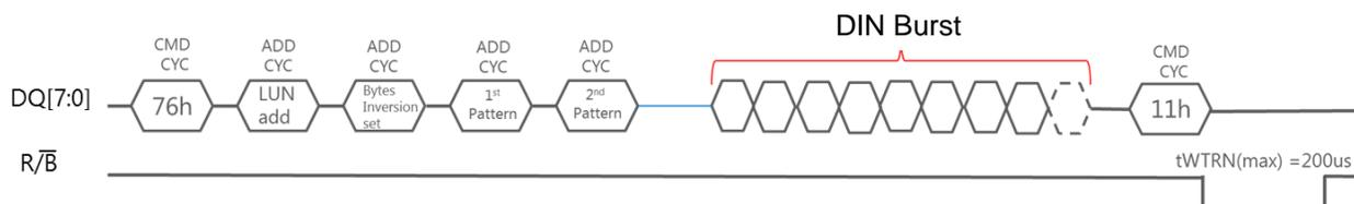
DIN Burst: Data Input with the same pattern specified in 3 address cycle wrapping around the data pattern length (16 or 32) for 1 full page
