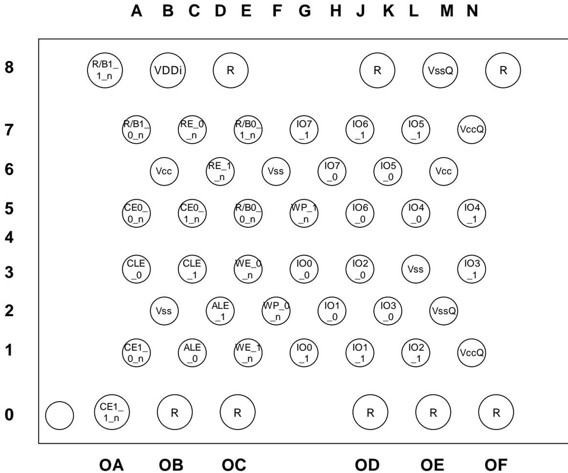
Figure 4 LGA pinout for 8-bit data access
