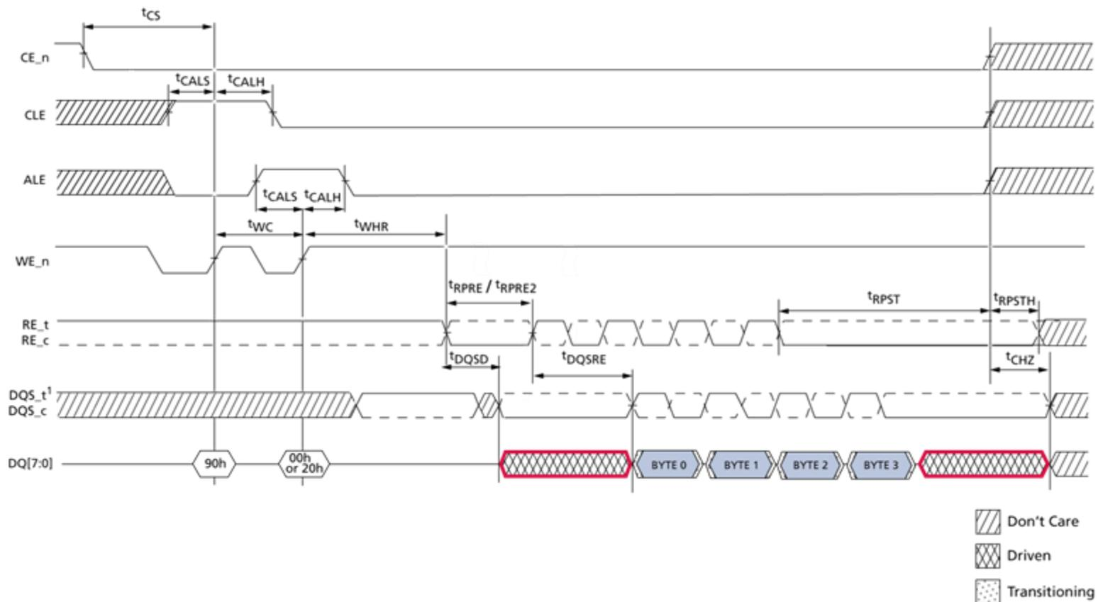
**Figure 89** Read ID command using NV-DDR2 or NV-DDR3 data interface
