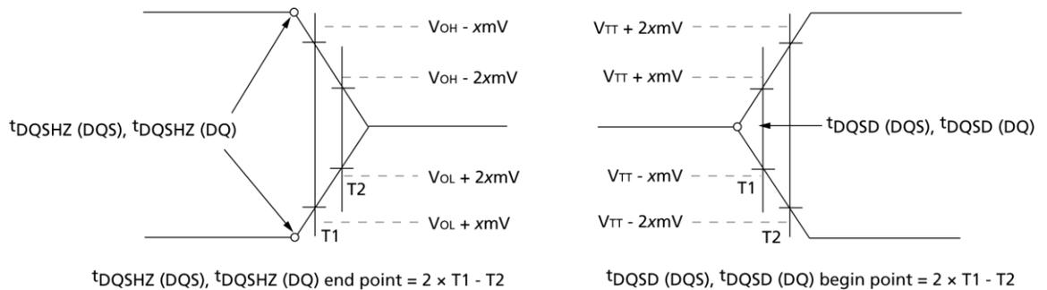
**Figure 150** Two point method for measuring timing parameters with tri-state condition
