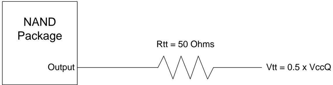
**Figure 40 Driver Output Reference Load**
