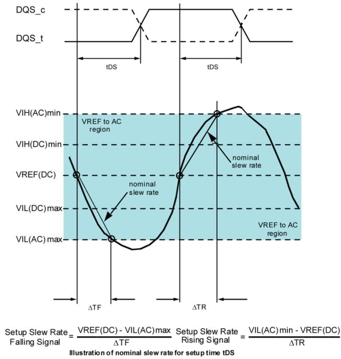
**Figure 46**      **Nominal Slew Rate for Data Setup Time (tDS)**
