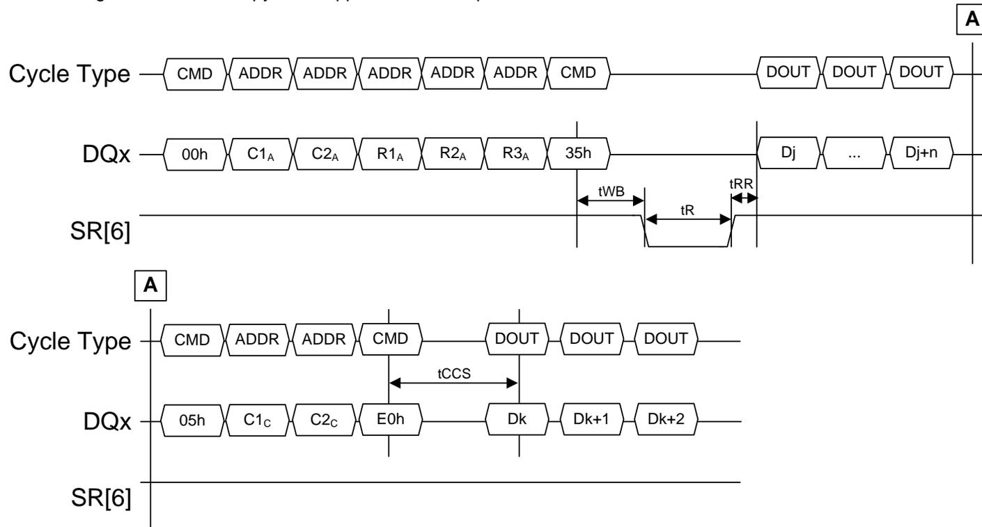
**Figure 106 Copyback Read with data output**
