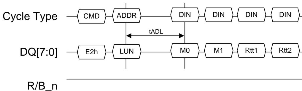
**Figure 116 ODT Configure timing diagram**
