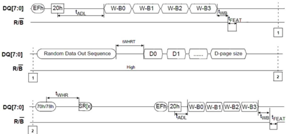
Figure 124 DCC (RE\_t/c) Training using Set Feature
