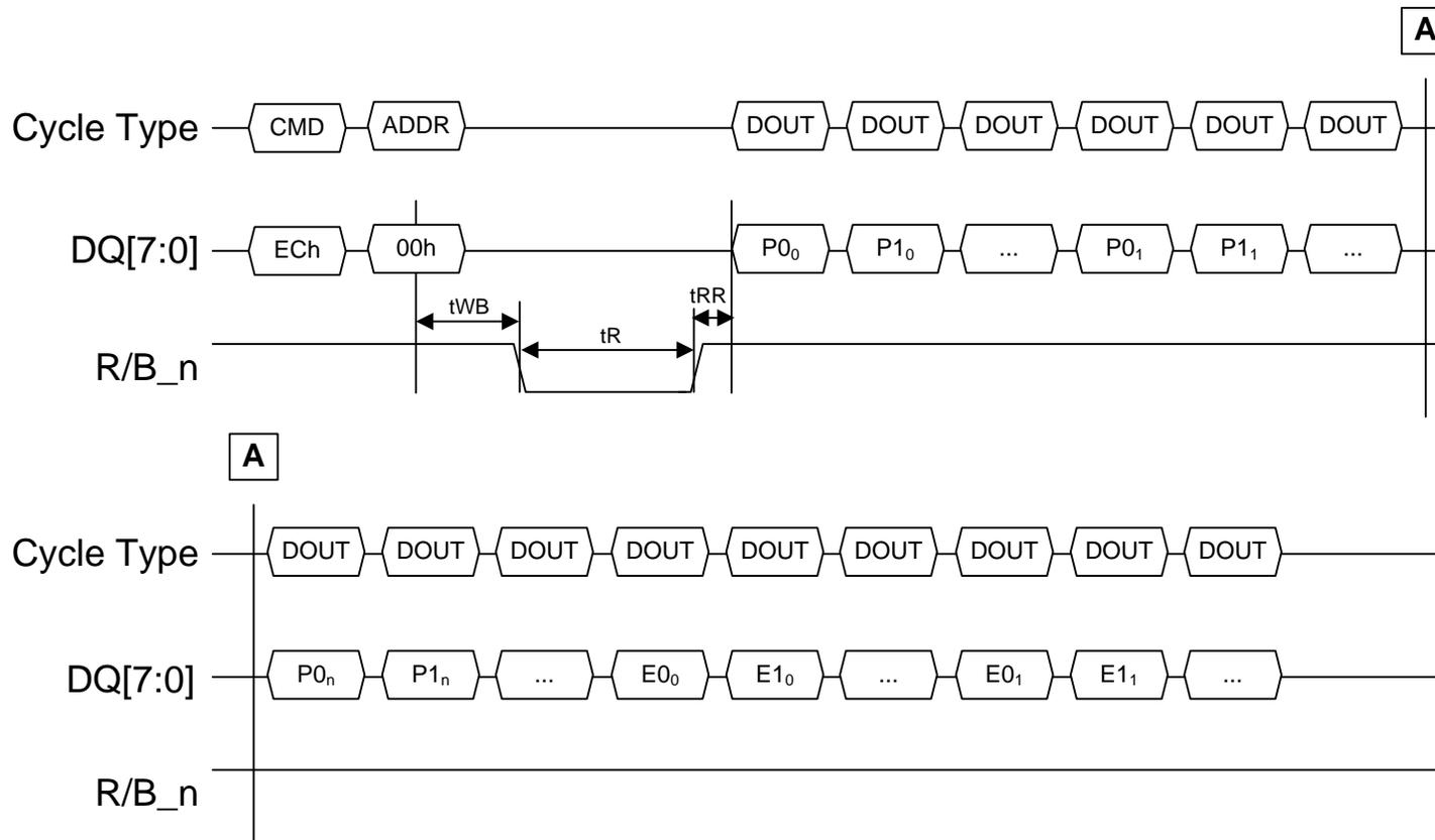
**Figure 90 Read Parameter Page command timing**
