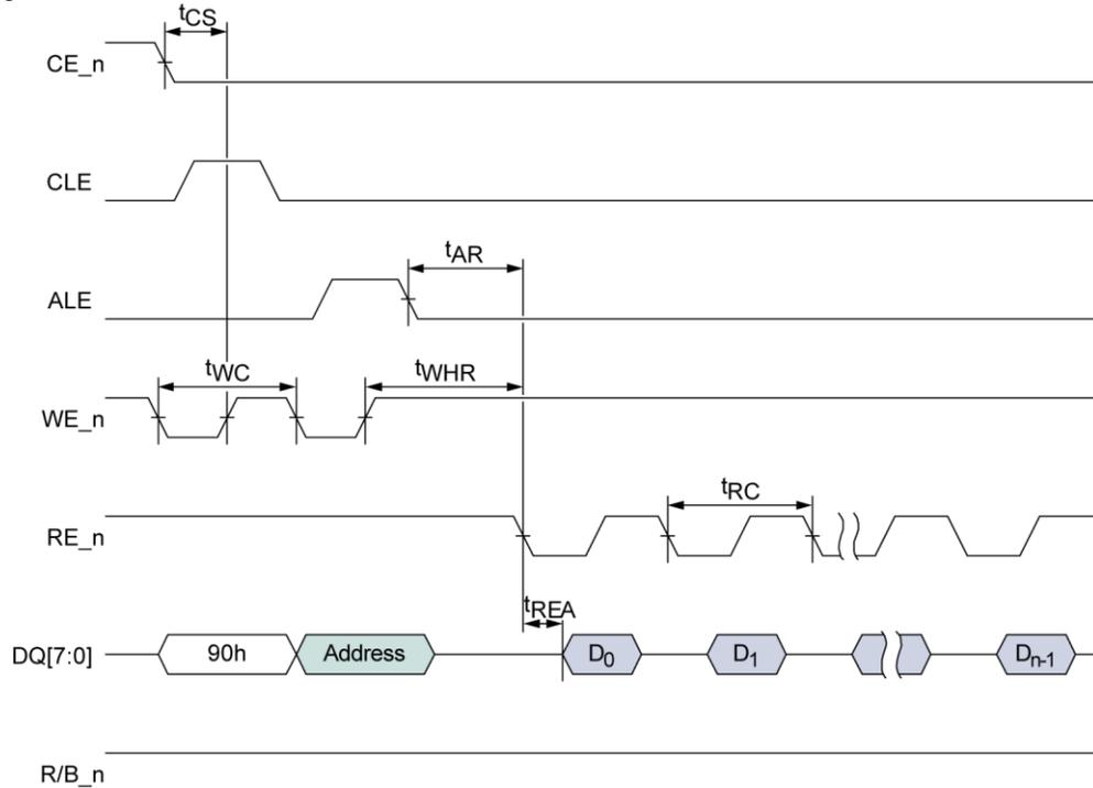
**Figure 87** Read ID command using SDR data interface
