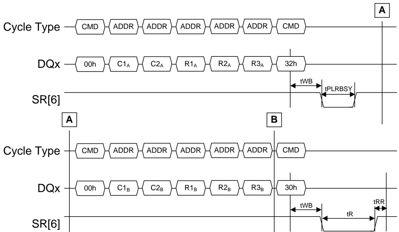
**Figure 140 Multi-plane Read command issue timing**
