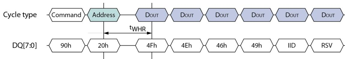
**Figure 85 Read ID timing diagram for ONFI signature**
