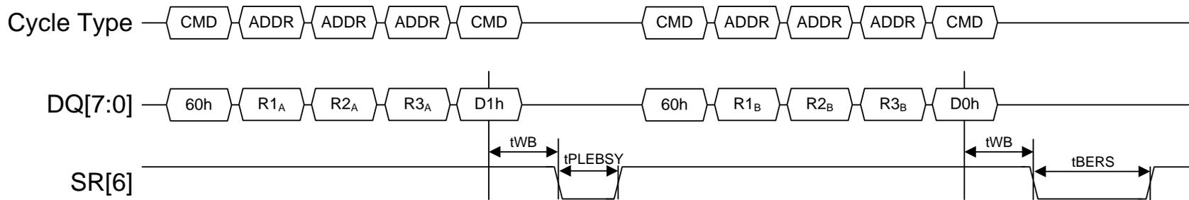
**Figure 138 Multi-plane Block Erase timing**
