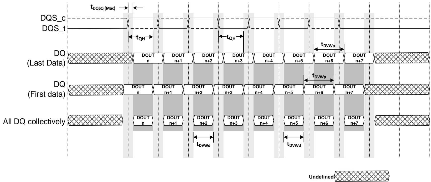
Figure 77 Data output cycle timing (after training)
