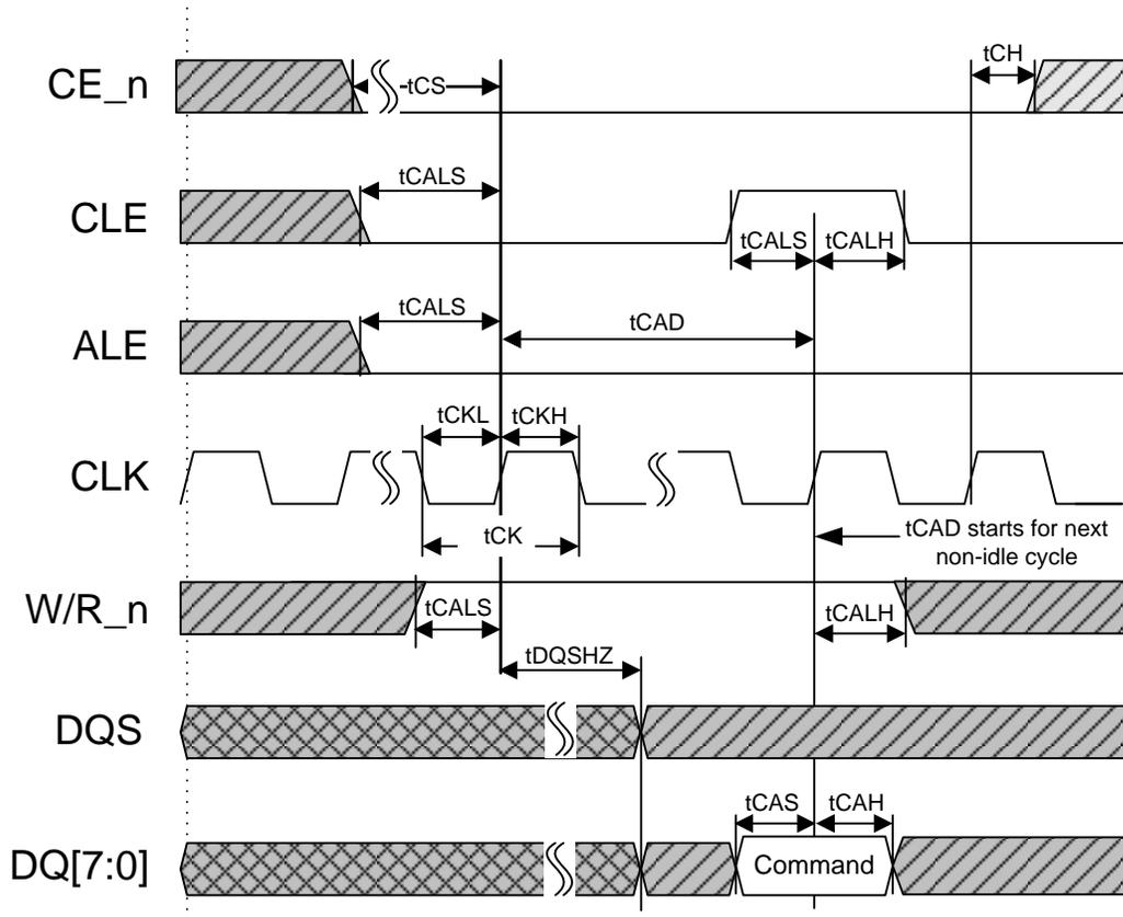
Figure 63 Command cycle timings
