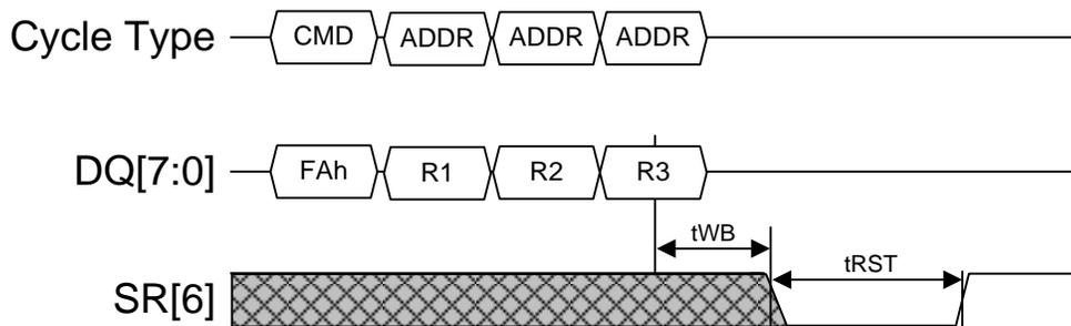
Figure 84 Reset LUN timing diagram
