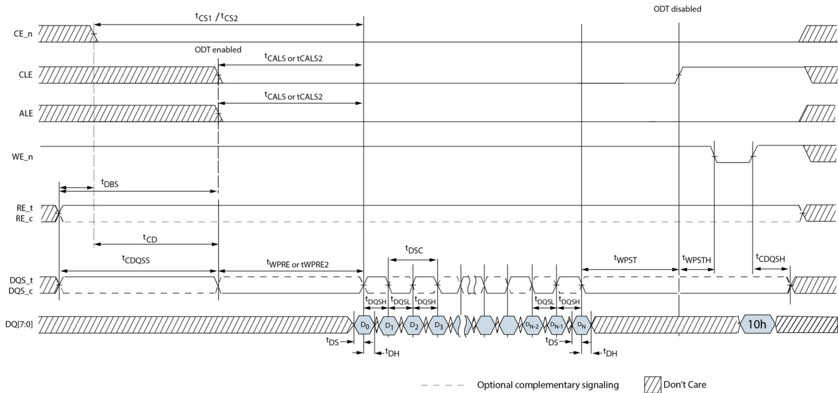
**Figure 74 Data input cycle timing (no training)**
