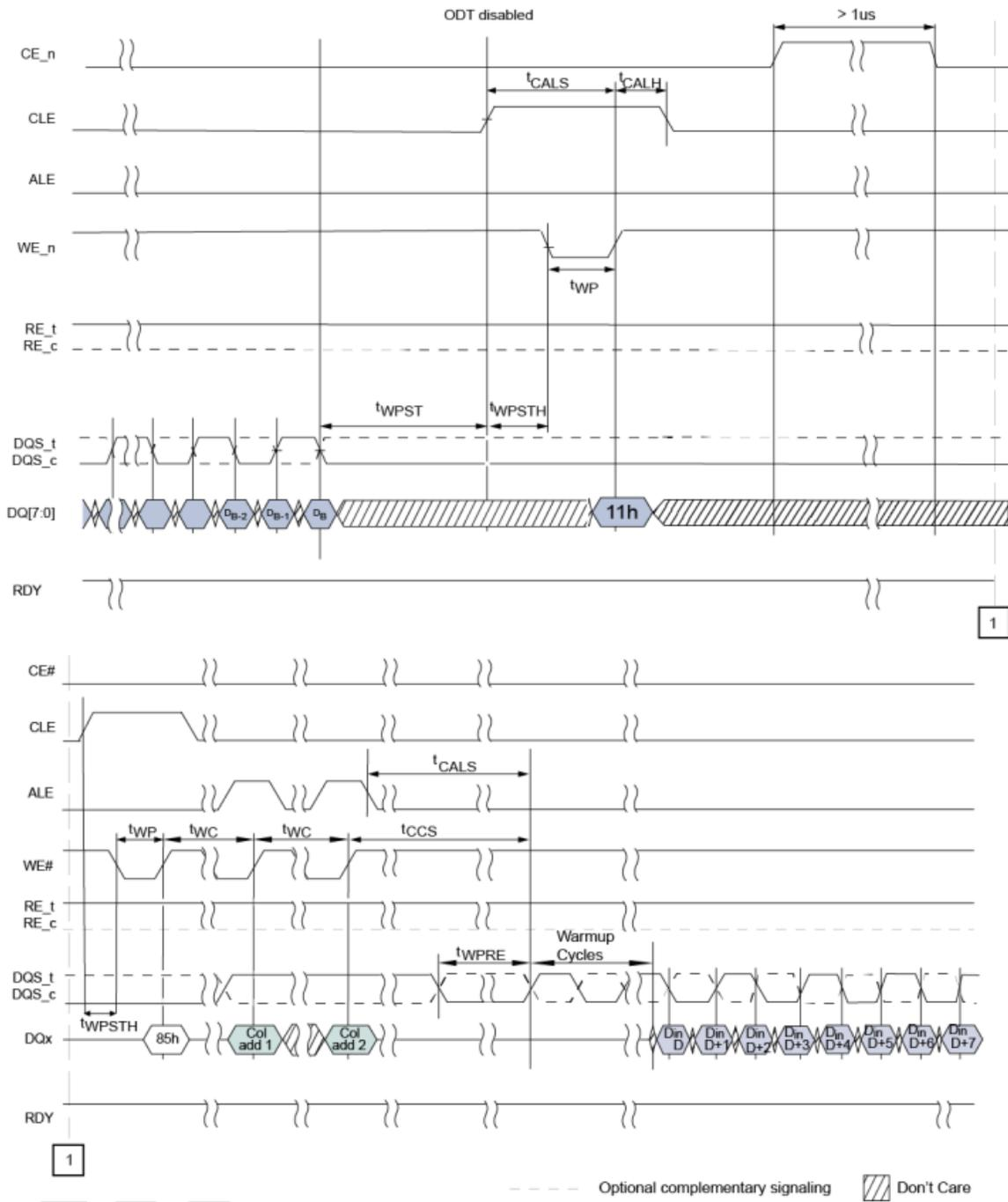
Figure 38 Example of Data Input Pausing for greater than 800 MT/s
