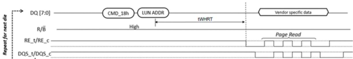
Figure 125 DCC (RE\_t/c) Training using Command (Optional)
